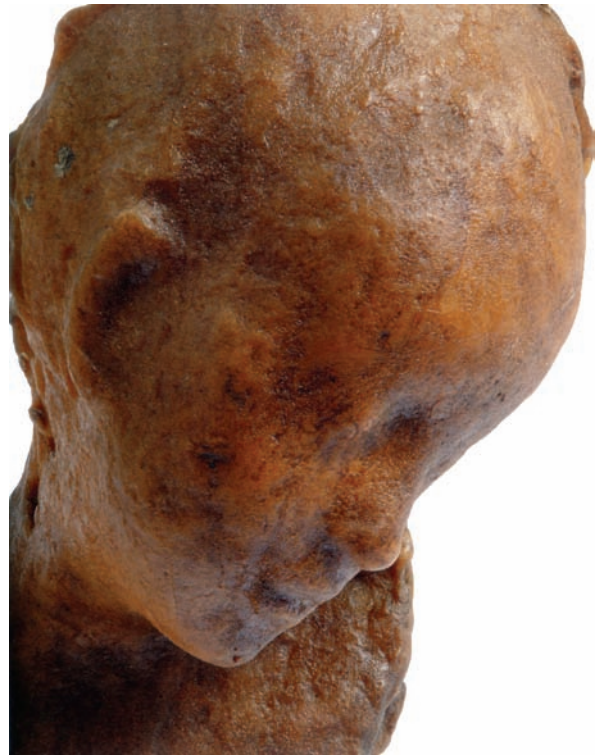
34. Another view of Fig. 30 showing pock and hole casting imperfections.
